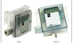
Accuracy <1% 70°C Max ambient Consumption at 0-10VDC 10mA 4-20mA 20mA nom pressure 0-10VDC Load 10ΚΩ 4-20mA at 24VDC 0.8K $\Omega$ Response time <20ms Ceramic/Silicon Media contact materials Max media temp 70°C Max pressure one side < 3mb 50mb > 3mb 100mb
