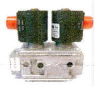
Technology: *Electro-Magnetic* Rated Voltage: 24V, *110V or 230V 50Hz* Fully Opened Power Rating: *15 - 46VA* Ambient & Media Temp range: *-10 - 60°C*
